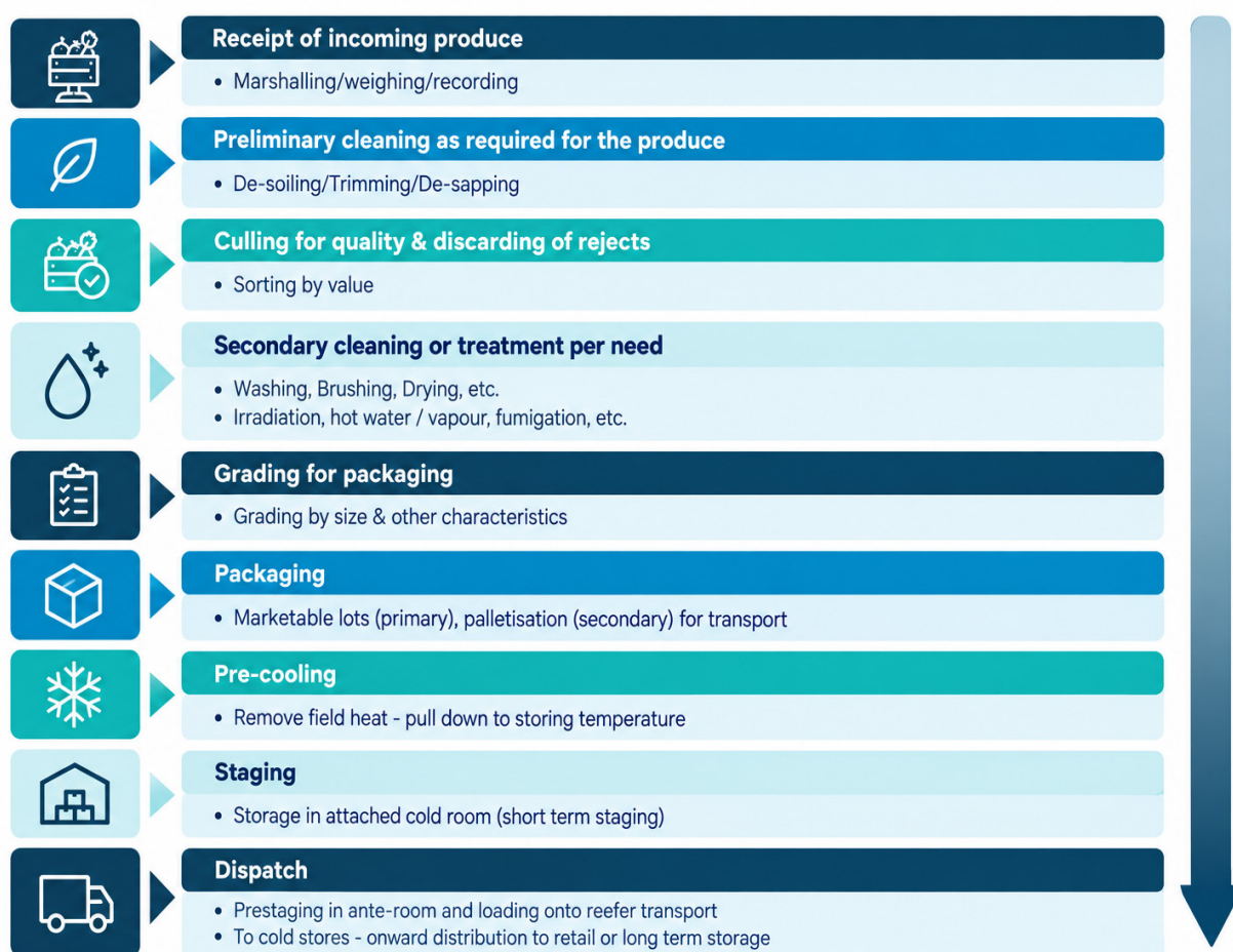
Figure 3: Typical produce flow in a packhouse
