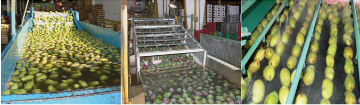
Figure 9: Initial fruit washing by tank immersion (left), spraying (middle), and on a brush bed (Right)
