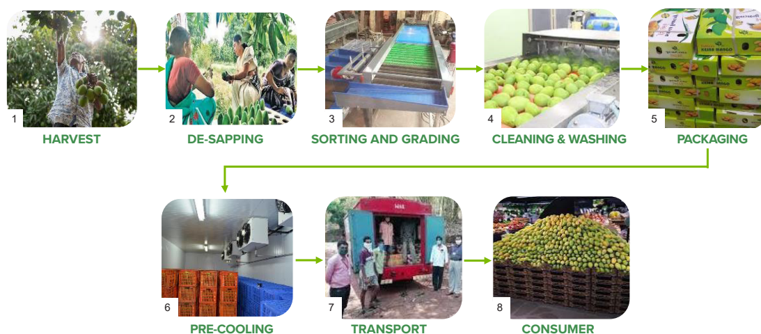
Figure 5: Process flow at Mango Packhouse for Local market
