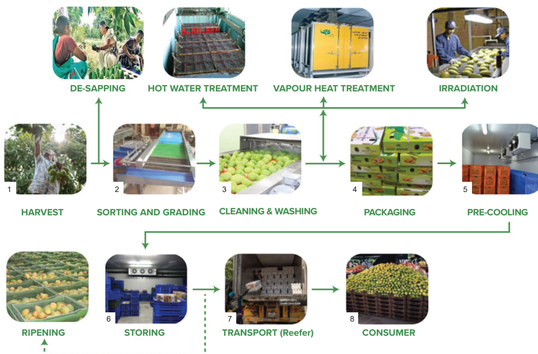
Figure 6: Process flow at Mango Packhouse for Export purpose/domestic premium market
